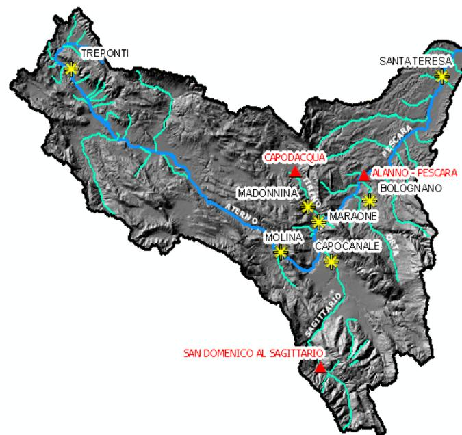
Figure 8. Spatial distribution of gauging stations for sediment load determination in Pescara river basin. The stations are represented by stars, whereas the red triangles show the position of the dams (compare with Figure 3).
