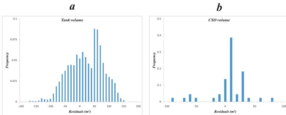
Figure 2. Distribution of the residuals between emulator and simulator: a) for the storage tank volume; b) for the CSO volume
