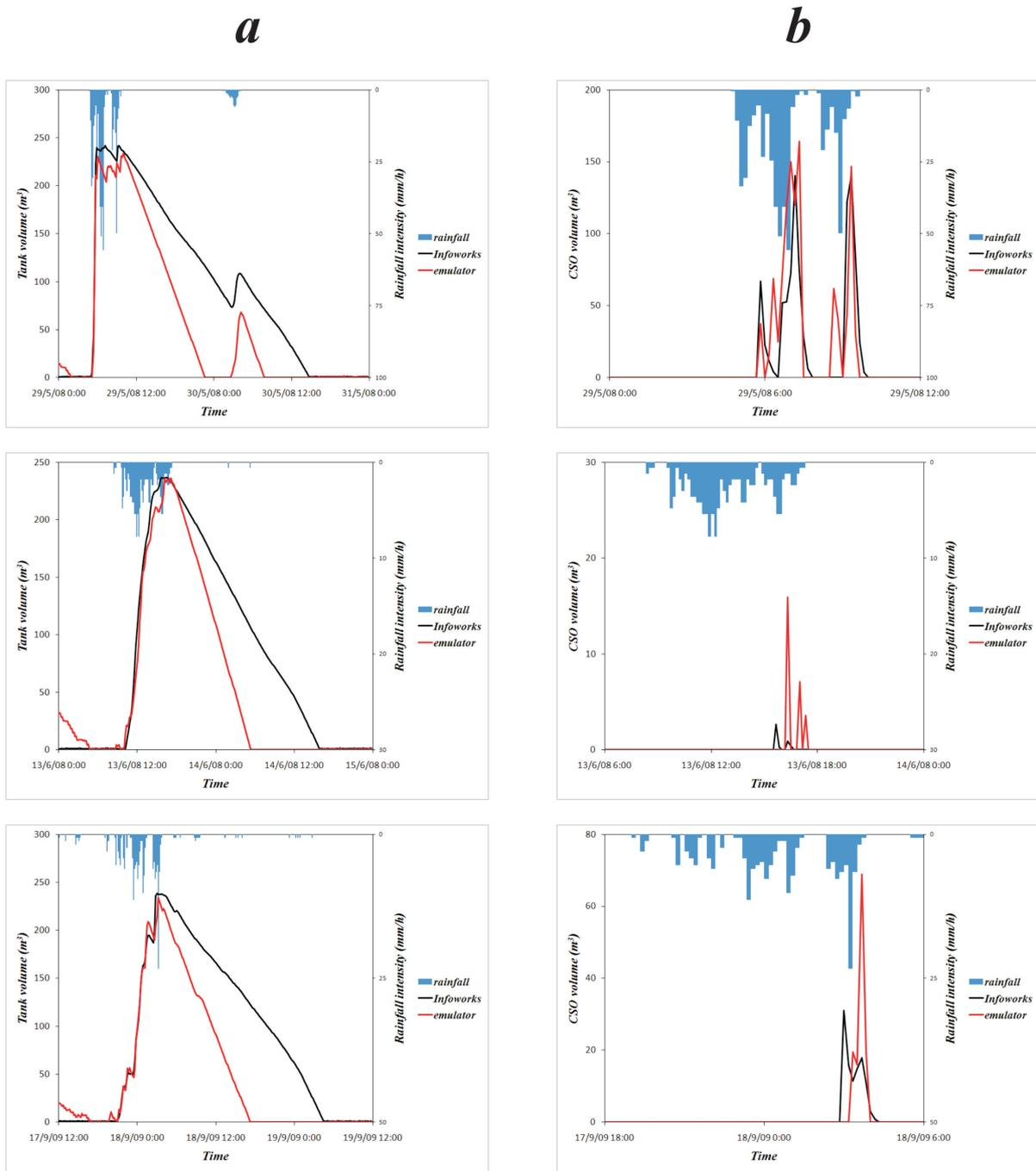
Figure 1. Comparison between emulator and simulator: a) for the storage tank volume; b) for the CSO volume.
