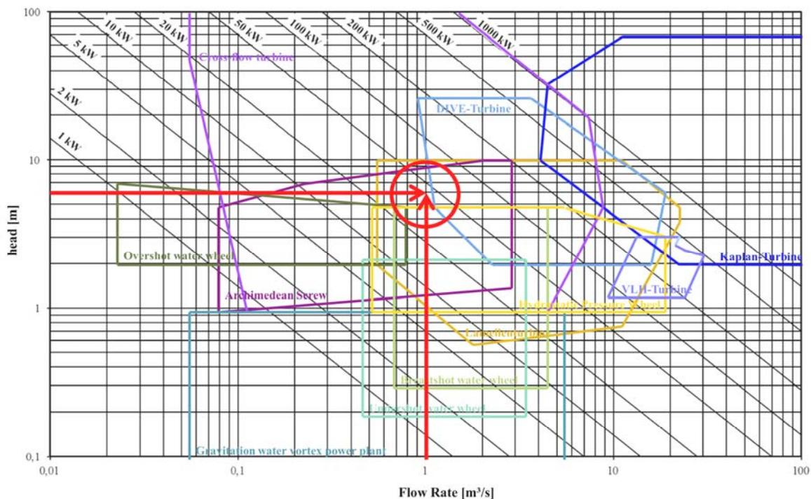
Figure 2. Application ranges of different small hydropower devices (Frehmann, Berger et al. 2013), red arrows mark the intersection for a given head of 6 m and a flow rate of 1 m<sup>3</sup>/s as an example
