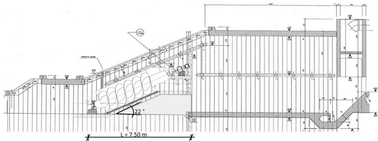
Figure 3. Possible position of the Archimedean Screw in the outlet of the WWTP Bottrop
