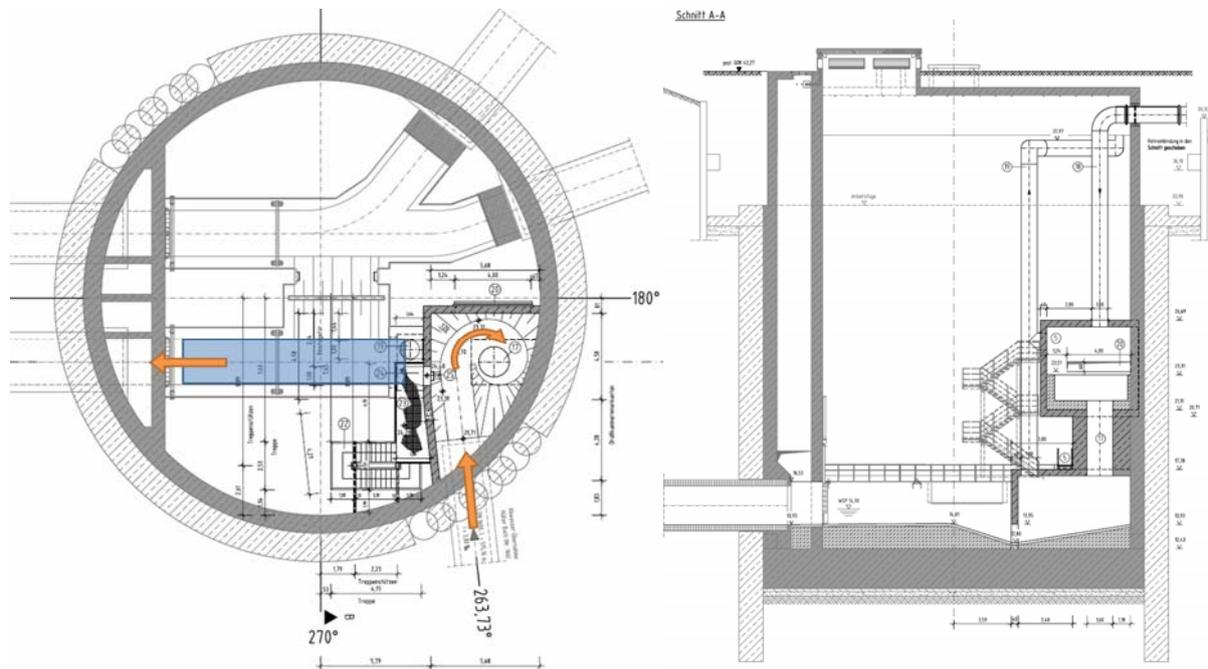
Figure 4. Typical manhole with vortex drop structure of the AKE in top view (left) and site view (right) with flow directions marked by arrows and a possible location for a hydro power device (rectangle)
