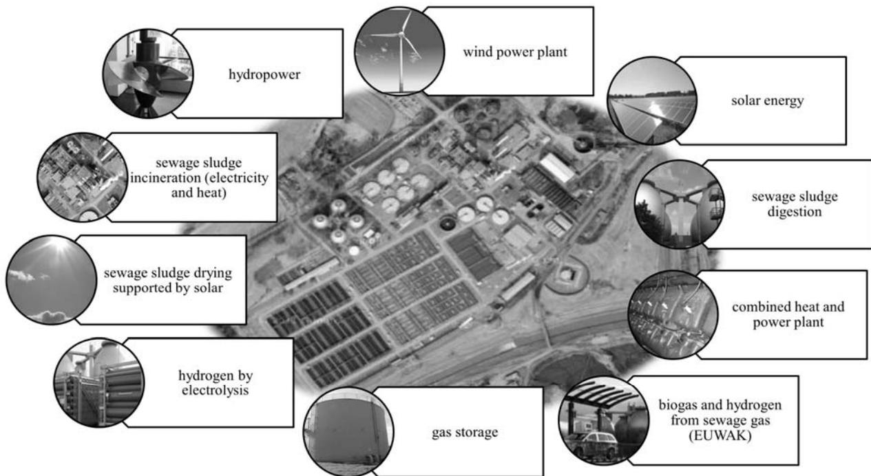
Figure 1. Elements of an integral energy management strategy on WWTPs, the "hybrid power plant Bottrop" (Stemplewski 2012)
