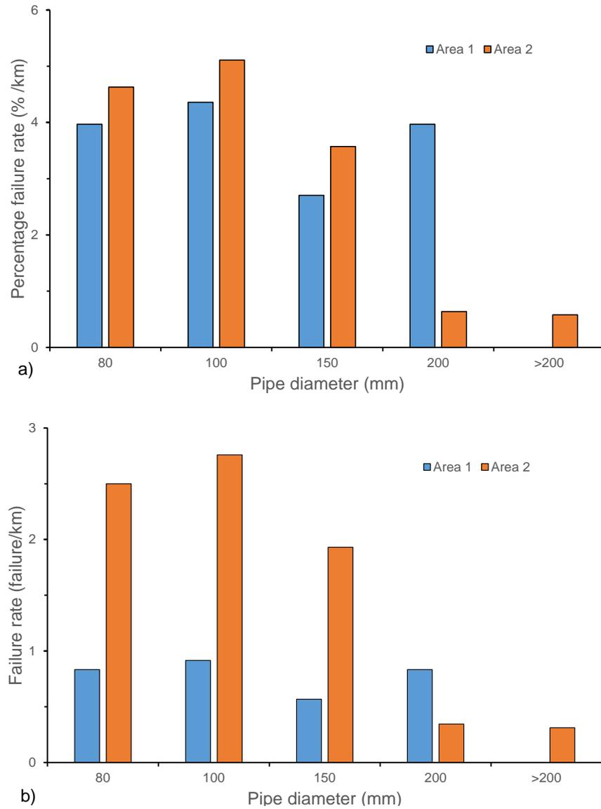
Figure 3. Comparison of (a) percentage failure rate and (b) failure rate for different pipe diameters.
