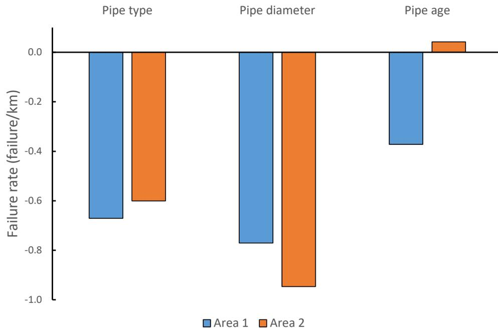
Figure 7. Coefficient of correlation between the failure rate and other influencing factors.
