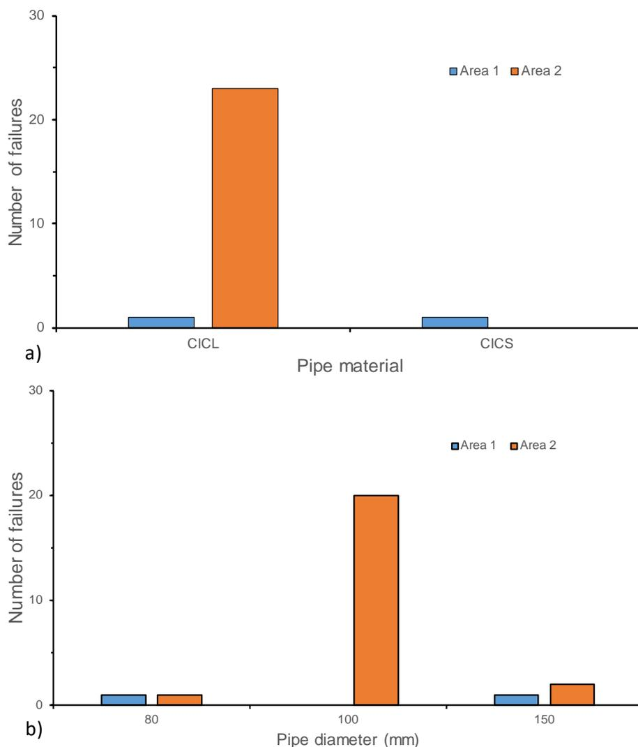
Figure 5. Comparison of 80-year-old pipe a) failure against built material and b) failure against diameter.
