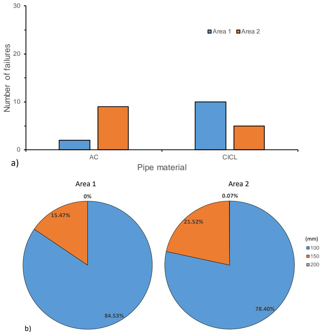
Figure 6. Comparison of 50-year-old pipe a) failure against material and b) failure against diameter.
