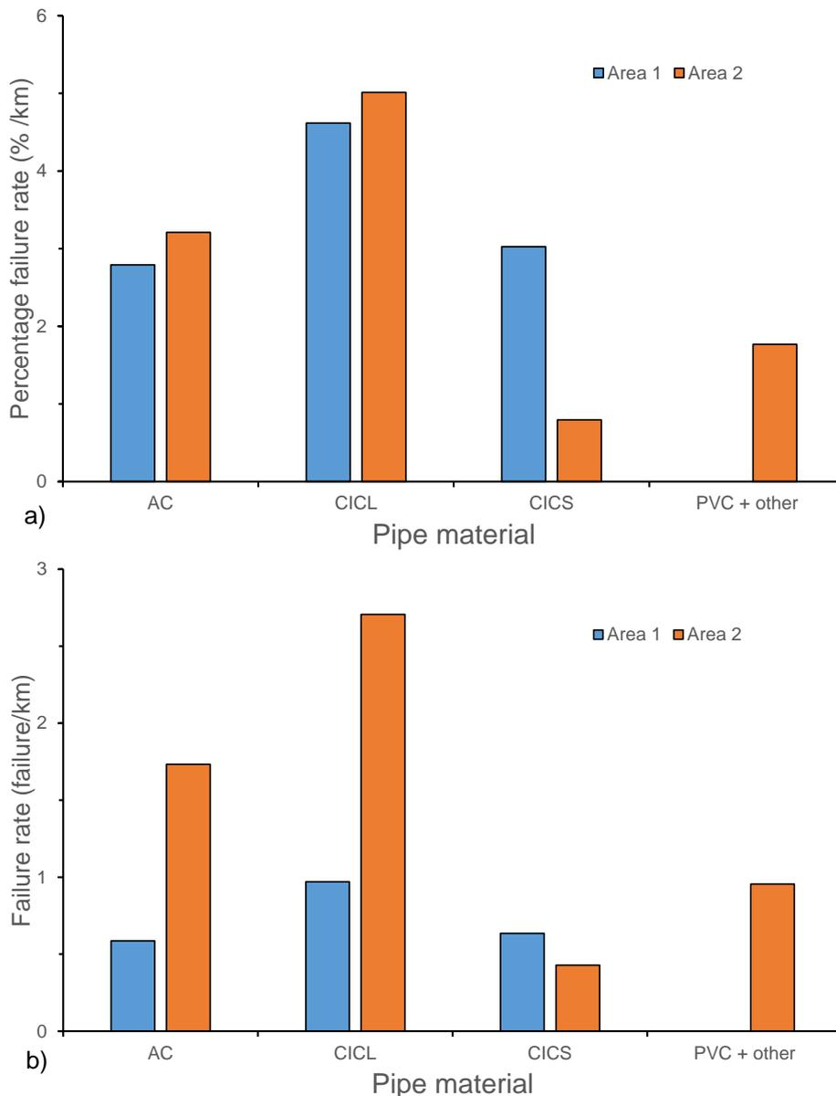
Figure 2. Comparison of (a) percentage failure rate and (b) failure rate for different pipe materials.
