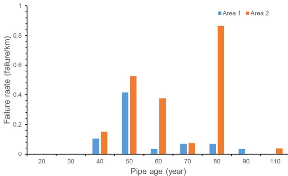
Figure 4. Comparison of failure rate based on pipe age.
