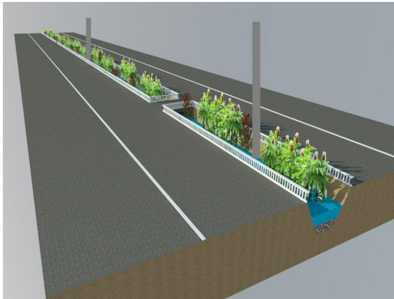
Figure 2. Schematic 3D illustration of the proposed stormwater recharge system integrated within the median of a roadway
